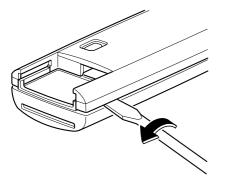
4. Remove the battery cap, then remove the battery.
